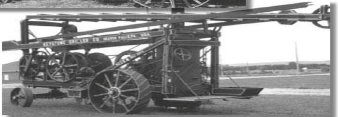
As time went on, more and more engines and boilers for cable tool drilling were sold as separate items (not mounted), and the layout was to have the steam engine fairly close to the derrick and the boiler farther behind. Both the mounted and the separated layouts were in use at the same time.
