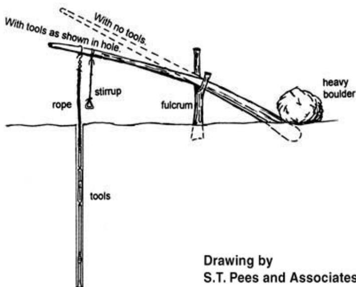
A lot of wells were started with the spring-pole. This method required strong legs and considerable time. The outfit was simple: a long pole, a weight to anchor the butt end, a fulcrum, stirrup, manila rope, oak rods, downhole tools including the percussion bit. More tools and other improvements would be added to the drill string as time went on.
